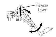
FIGURE 6.6 Raising/Lowering Elevating Front Riggings
